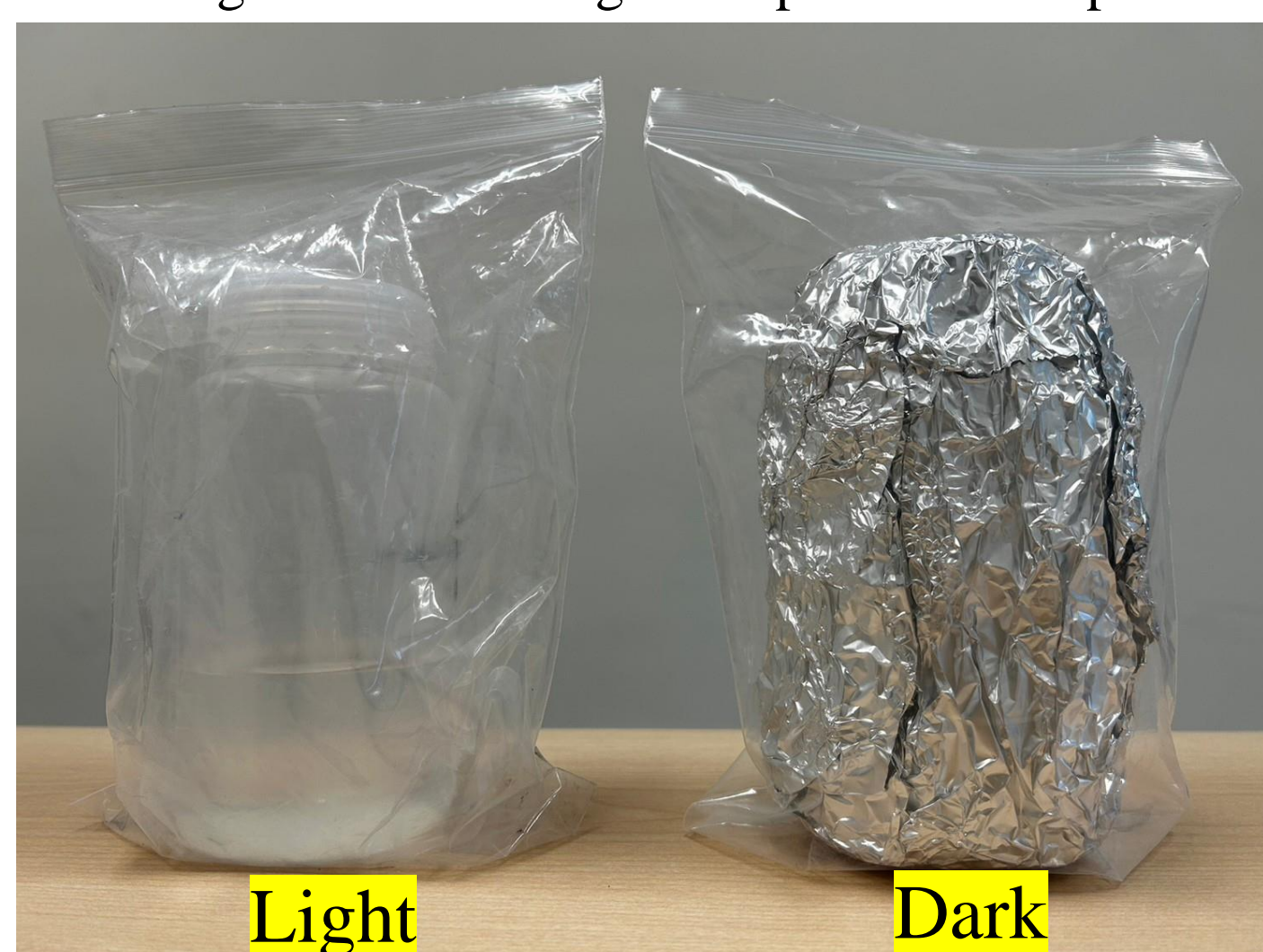
Figure 4. Illuminated (Light) and non-illuminated (Right) PFA bottles.
