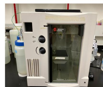
(Left) Use Beckman Coulter Multisizer to measure cell numbers and specific growth rates.
